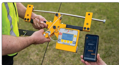
Quick Check "T" shown with Test Bar and phone APP
