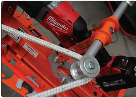
Safety Rope Diversion allows Operator to stand out of pulling line
