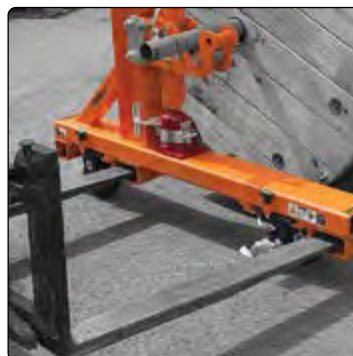
RBJ20K pockets for forklift tynes
