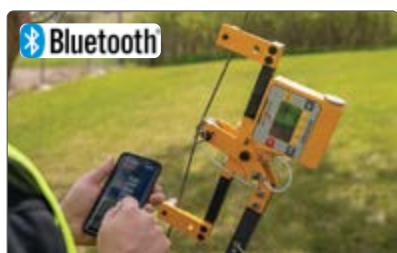
Quick Check "T" shown testing tower guy with phone APP
