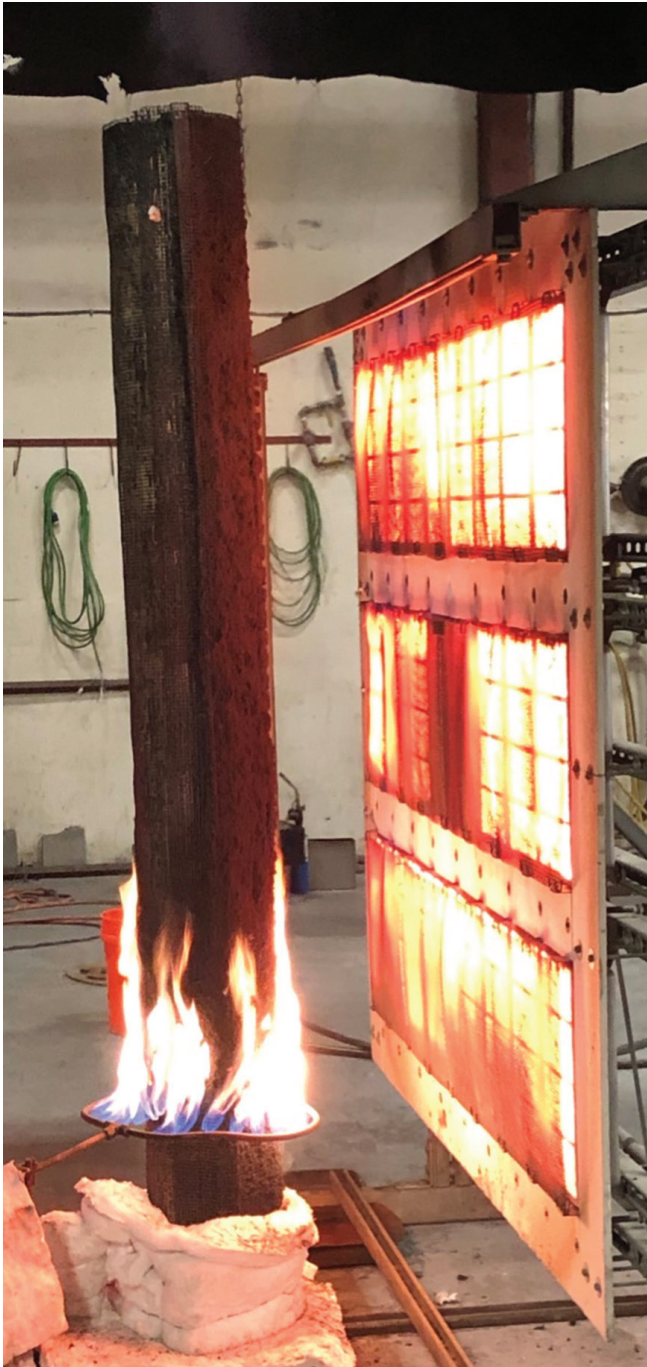
Image 3 Simulated Forest Fires test the real-world performance of FireMesh in protecting structures
