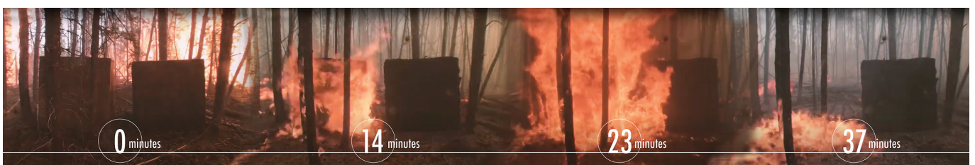
Image 2 Radiant Heat Panel set to 980°C during Testing at the Western Fire Centre in Washington.
