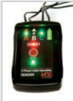
LED lights indicating connected and shorted phases
