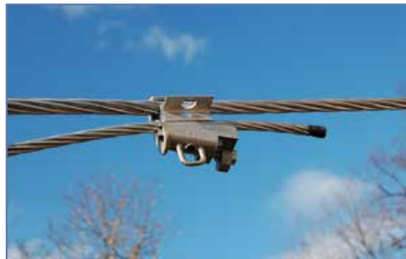
6) The Shear Head Bolt will break off at 12-15 [ft-lbs]. of torque which yields approximately 3000 lbs. of connecting force on the conductor.
