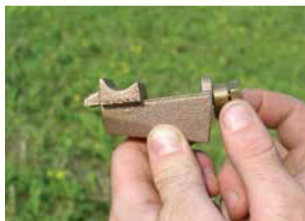
1) Withdraw drive screw to end point of wedge as shown.
