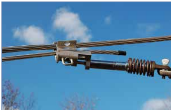
5) Lock the Connector by driving the Shear Head Bolt with a standard hex drive device.
