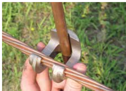
3) Place conductor designated by markings on cable nest within "C" body.
