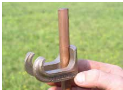
2) Place "C" Body around conductor
