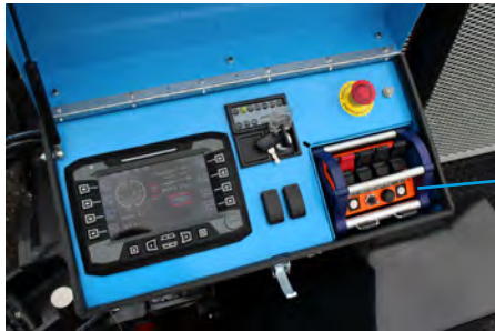
7" COLOR DISPLAY gives all of the information you need during the pull
