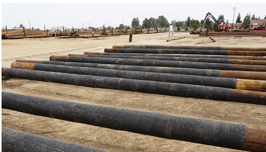
Poles in a yard pre-wrapped with FireMesh ready for install
