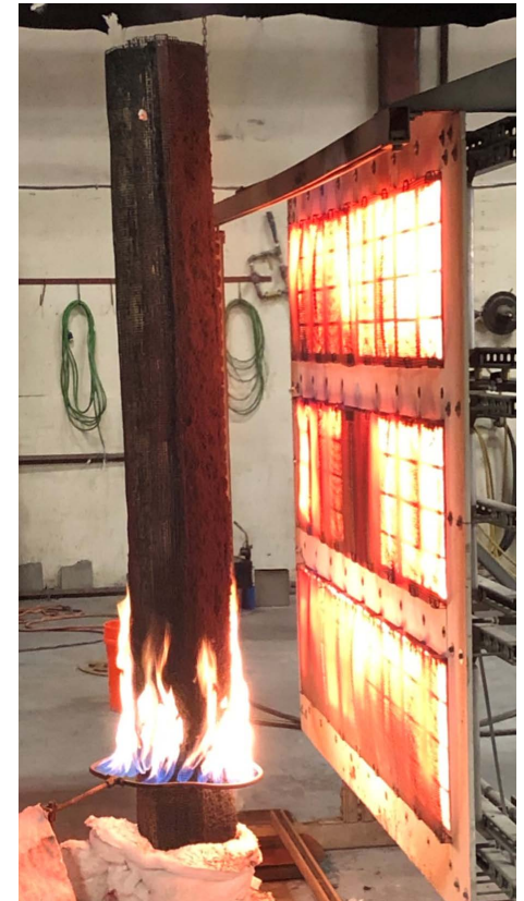
Radiant Heat Panel set to 980°C during Testing at the Western Fire Centre in Washington
