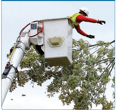
Foam filled for added electrical safety protection
