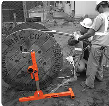
Separate Stands and height adjustment allows for use on uneven ground
