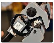
Unique, low-friction V-jaw provides precise & accurate clamping.
