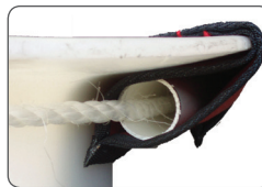
Apron folds over bucket lip and ties underneath using rope & conduit
