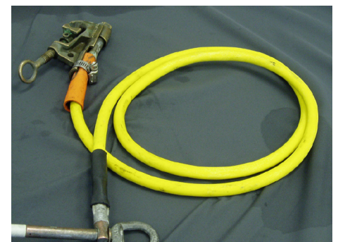
Cleaned Earth Lead
