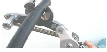
2. Set the cable between the blade, and set the pawl lever to cut side. The blade closes automatically.
