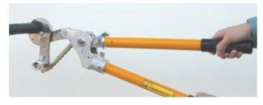
3. Operate handle and repeat. This will cut the cable. Repeat Step 1 to release.
