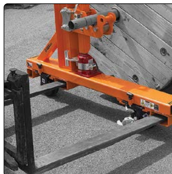
RBJ20K pockets for forklift tynes
