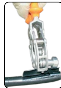
Stripping of Sheath
