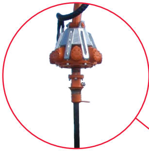
Lifter Borer Drive Motor & Kelly Bar, which couples with the Kelly Bar Adaptor & assembly as below
