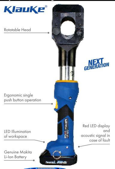
Ideal for cutting ACSR, Cu, Al and St round cable, armoured, structural steel + stranded copper cables
