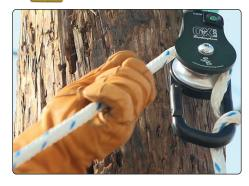
Replace many of the older style pulleys and tackle with the lighter Ox Block system, making rescue, lowering and raising and snubbing workloads easier
