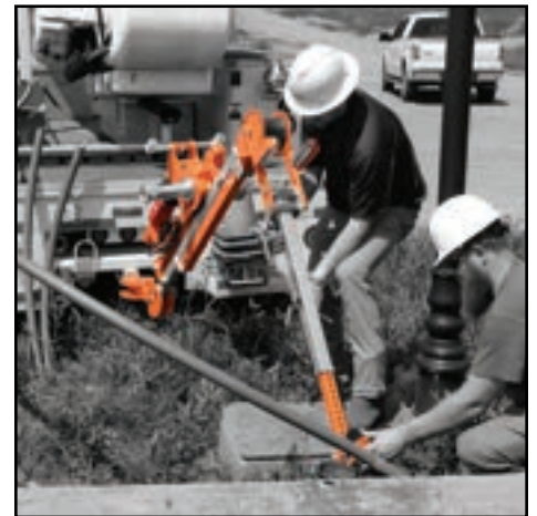
Boom articulates for underground applications.
