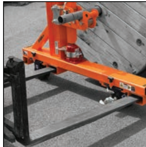
Lifting can be done from all four sides with forklift.
