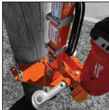
Engagement teeth bite into the pole.
