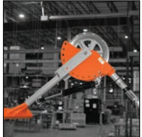
Hydraulic adjustment of extensions.
