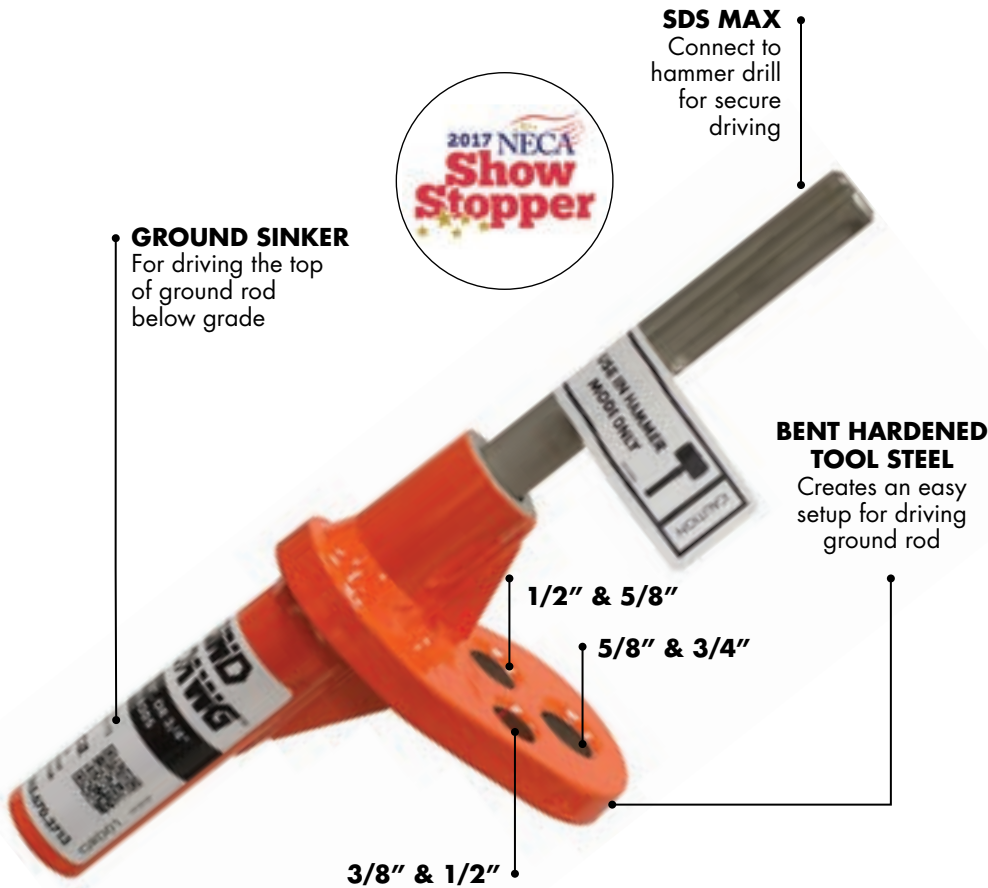
Safely drive rods from ground.
