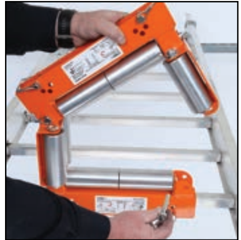
Two snap together in seconds to guide trapped conductors.
