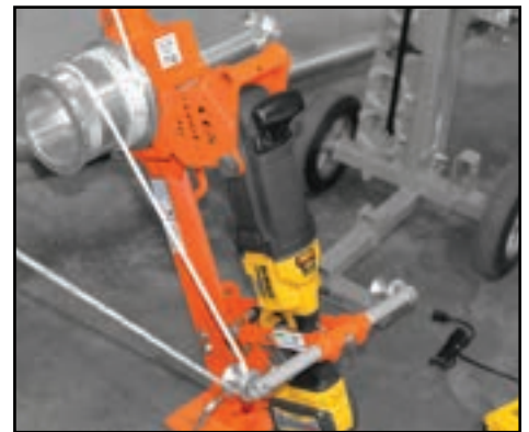
Built-in rope engagement capstan switch.
