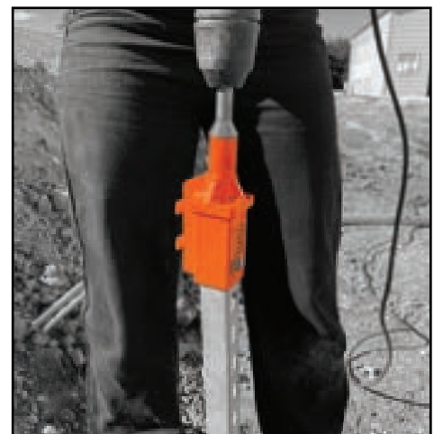
End receiver for driving from the top.
