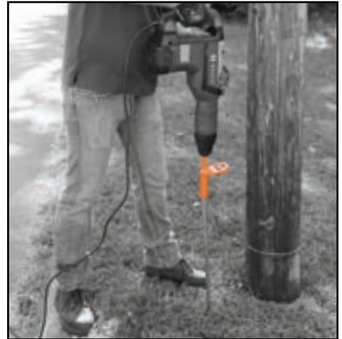
Tool locks into hammer drill.
