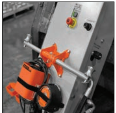
Control your pulling force using the output torque limit dial.
