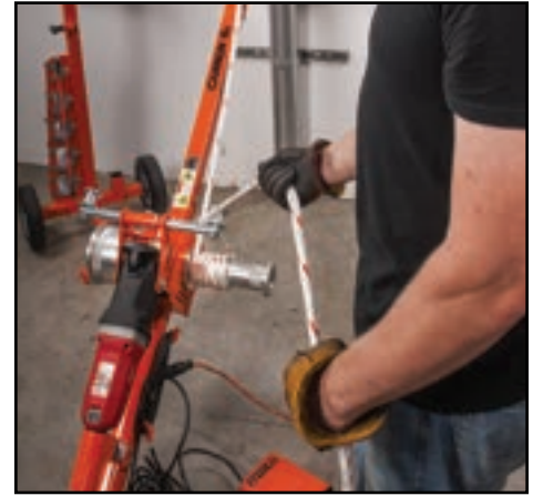
One pop pin removes the 6K from cart. Shown pulling on the 6,000 lb. capstan.
