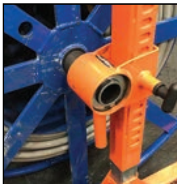
Axle-less on steel reel with 2" arbor holes
