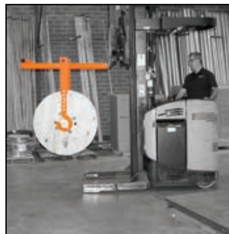
Load hanging center can be moved for heavy loads.
