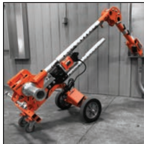
Extra extensions store on puller when not in use.
