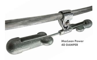
Vibration dampers are typically installed along the length of the transmission line at regular intervals. They work by absorbing some of the energy of the oscillations, which reduces the amplitude of the vibrations and the stress on the conductors. This helps to prevent damage to the conductors and ensures the safe and reliable operation of the transmission line.
