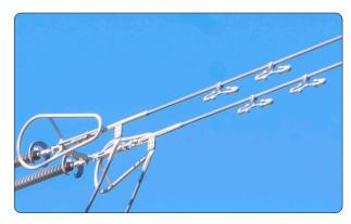
4D dampers are suitable for use on all conductor and earth wire constructions including ACSR, AAC, AAAC, AAAC 1120, HDC, galvanized steel (SC/GZ), Aluminium clad steel (SC/AC) construction, and Optical fibre ground wire (OPGW); sizes are available to cover the range of sizes from 7.5mm to 45mm.
